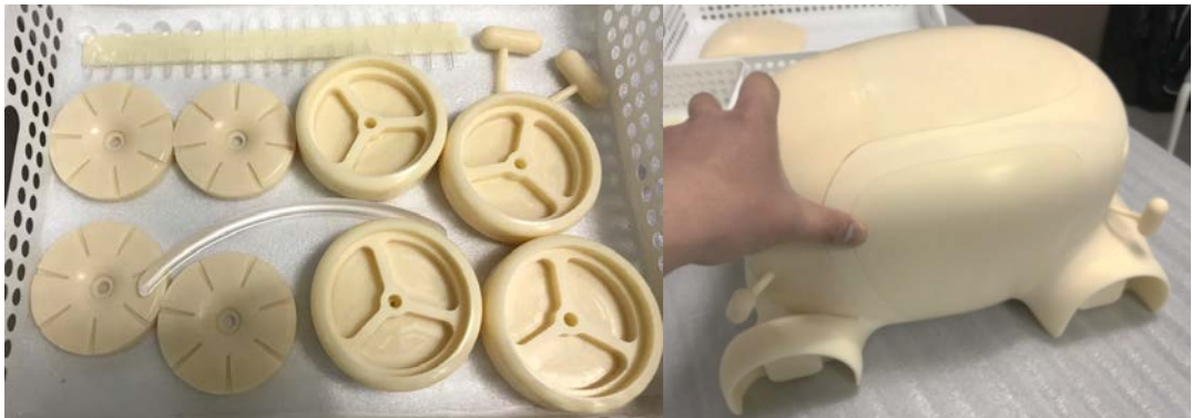
Figure 82. Left is 'Parts made with CNC', Right is 'Assembled Model'
