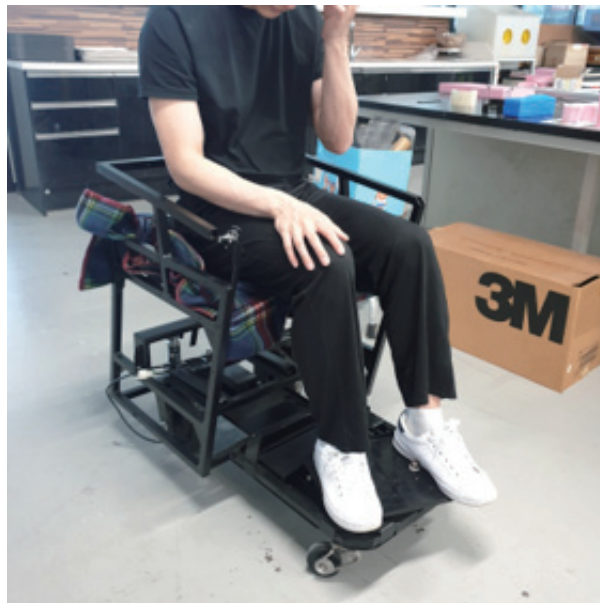
Figure 12: Prototype of sliding footplate
