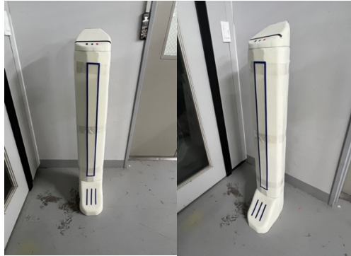
Figure 11: Low fidelity prototyping test with isofoam
