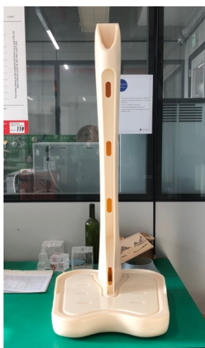
Figure 23: The final model through CNC machining
