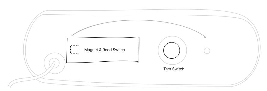
User can turn it on or off by using the strap with a magnet.
